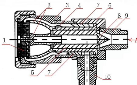
**Figure 1 Schematic of Co-extrusion die**
