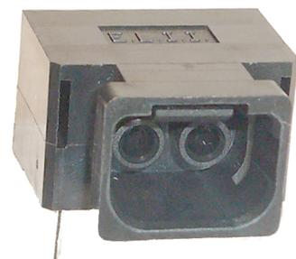
Compliant with the International Electrotechnical Commission standard (IEC 61754-21), the company's new connector system uses RCLED-based light sources from Firecomms, Ltd. that operate at 100 Mbps (125 Mb) for 100 meters, and 200 Mbps for a distance of 50 meters. With a maximum insertion loss of 3.0 db with 500 cycles of durability, this new connector system uses plastic optical duplex cable assemblies of up to 100 meters that also are provided by Electronic Links.
