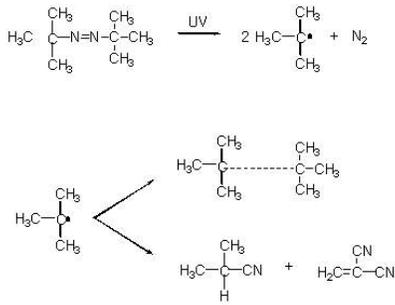
Fig 1. Azo compound decomposition by UV energy
