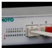
Installing Plastic Optical Fibre is as simple as cutting it with a knife, plugging it into the connector and locking the connector into place.
